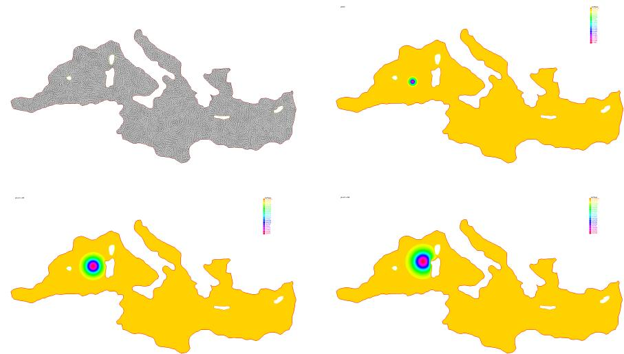
**Water Quality Model :** Concentration of pollution  $n$  is the number of outlets,  $f_j = q_j \rho_j^i$ , where  $q_j$  is the river flow rate at outlet  $j$  and  $\rho_j^i$  the partial density of the substance  $i$  at the reject point  $j$ .  $\delta_{p_j}$  is the Dirac measure at the outlet  $p_j$ .
